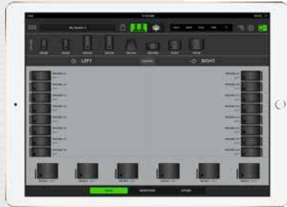
Rig View Discovery, grouping, and configuration of all networked loudspeakers
