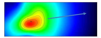
Above, an array with LF correction to shift the low-frequency energy towards the majority of the audience (on the right side of the venue), reducing excess bass energy behind the array and in the side audience areas. No physical changes have been made to produce this benefit – it is an inherent component of how Adaptive Systems work.
