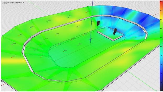
In a typical 15,000-seat arena, a system of 20x Anya, 12x Anna, and 12x Otto will provide consistent 270° coverage, employing two arrays with main columns of 10x Anya modules each and outfill columns of 6x Anna modules each. Low frequency support is supplemented by two arrays of Otto, 6x modules each. Predicted SPL is a consistent 105 dBA, +/- 2 dB.
