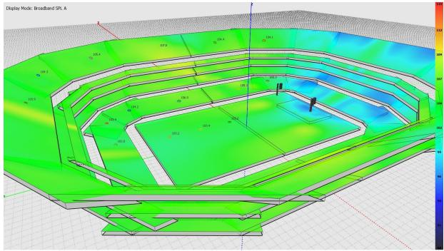
This example illustrates a large stadium with the stage configured at one end, and seating wrapping around 270°. Each array consists of two columns: one of 18x Anya modules for the 'long-throw', and another column of 14x Anna modules for outfill. Even with a large throw distance differential between columns, SPL is remarkably consistent. Low frequency support is provided by 24x Otto.
