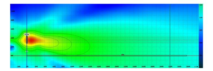
Finally, we see the result when the maximum number of Anya enclosures is suspended (maintaining a 10:1 design factor). This 18-module column of Anya produces an extremely tight vertical pattern at 125Hz across this listening area. If directivity at lower frequencies is required for the application, array length must be considered.
