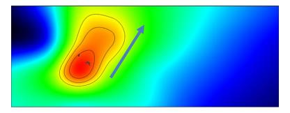
Above, an array without LF correction – Low-frequency energy is directed through centerline of array, diagonally. This is the 'natural' response of this array geometry.
