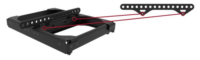
2. Place flybar assembly on top of SB818P|F and use M8 X 30 bolts w/flat and lock washer to rig front and rear positions.
