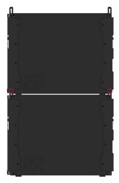
3. To add KF810P, start by placing frame on top of SB818P|F array, and securing front and rear rigging with M8 x 30 bolts w/flat and lock washers. "Z" hole needs to be orientated towards the front of intended array.
